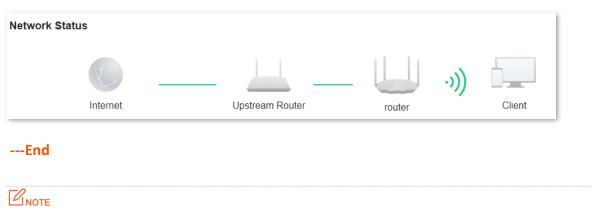
If there is another network device with the same login domain name (**tendawifi.com**) as the router, log in to the upstream router and find the IP address obtained by the router in the client list. Then you can log in to the web UI of the router by visiting the IP address.
