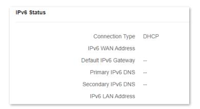
This part is only displayed when the IPv6 function is enabled. You can view the information on IPv6 connection, including connection type, IPv6 WAN address and IPv6 LAN address.
